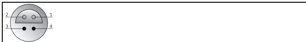
Pin assignment (front view)
